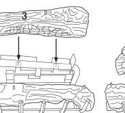
Figure 42 - Installing Log No. 3
